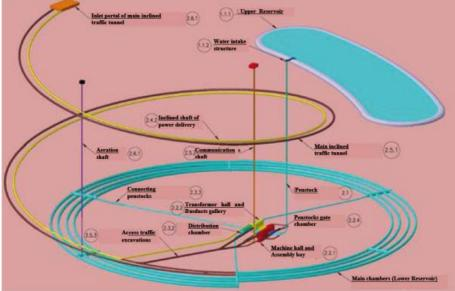
Figure 4. Scheme of a 1000 MW pumping plant with a spiral shape gallery underground reservoir [10]
