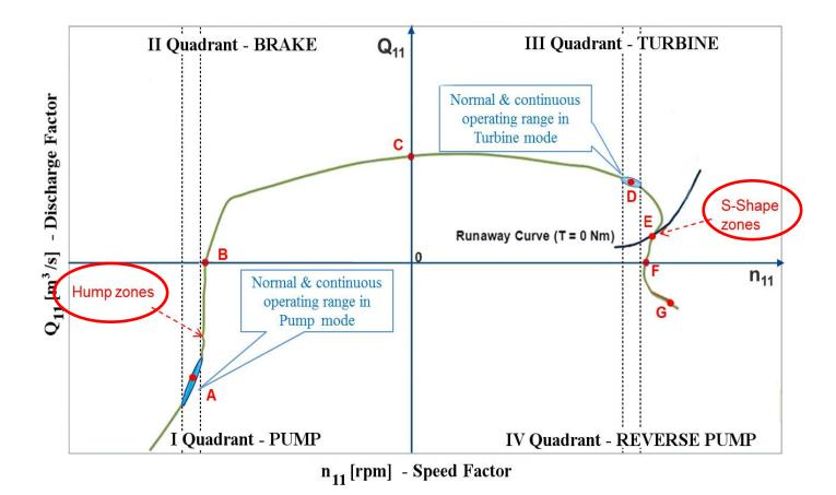
The capability of PHES plants in providing grid services is mainly limited by unstable behaviours both in pumping than in generating mode:
