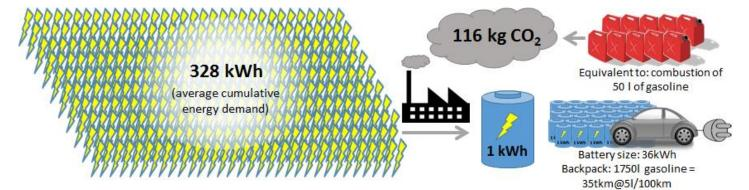
Figure 2. Average cumulative energy demand and CO2 emissions for manufacturing 1 kWh of lithium-ion battery. Own picture, data from [2] http://www.eera-set.eu/eera-joint-programmes-jps/energy-storage/
