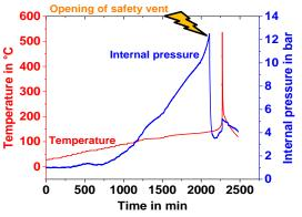
Figure 3. Temperature and internal pressure variation during thermal abuse of an 18650 cell [2].
