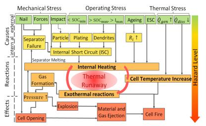
Figure 1. Causes and effects of thermal runaway in electrochemical cells during normal use, abuse or accidents.
