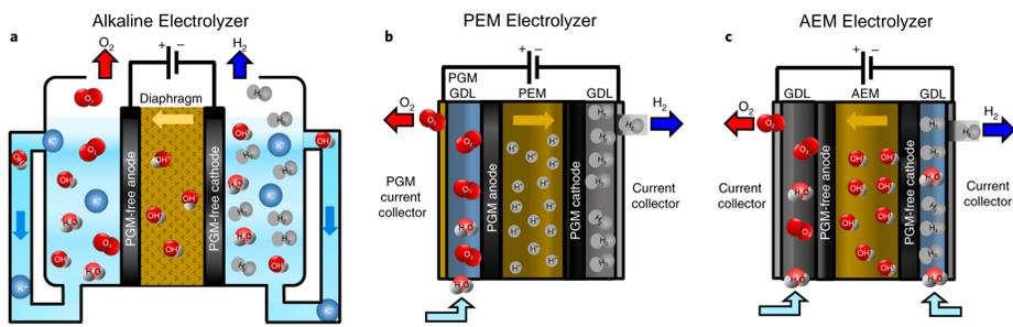
Figure 1: Operating principles of Alkaline Electrolyzers (a), Proton Exchange Membrane Electrolyzers (b) and Anion Exchange Membrane Electrolyzers (c).[6]
